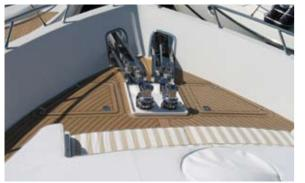
**Flexiteek is supplied** ready to lay. All our decks are custom made from templates for each project. We supply them in one piece ready to glue down, complete with margins, hatches and deck details.
